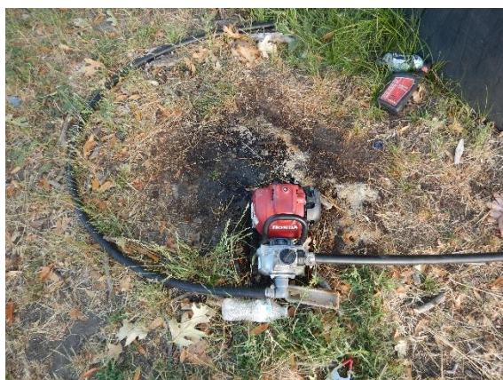
Photo 3: Uncontained portable pump near GH1-3 and T1
